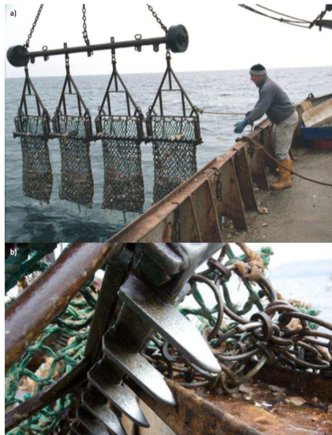
Figure 3.6: Images showing Newhaven dredges (a) Four spring toothed Newhaven dredges showing tooth bars, dredge frame and nets and the rubber wheeled towing bar. (b) Close up of the dredge teeth. Images taken from Howarth and Stewart (2014)
